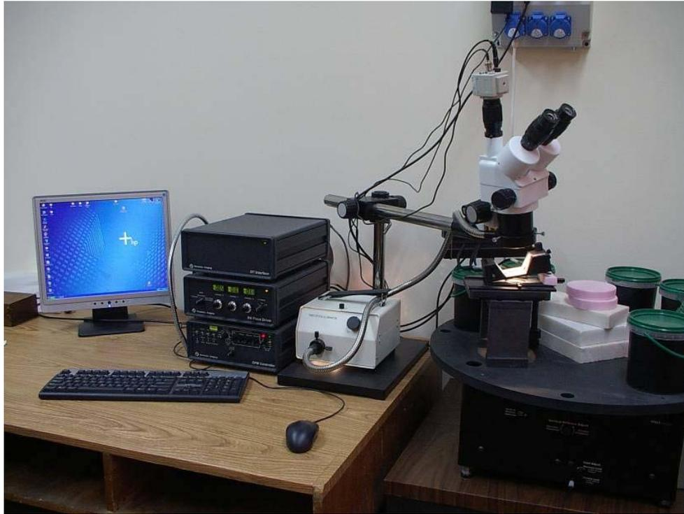
Figure 1. Nanonics Imaging Multiview 1000 AFM and Academia optical microscope
