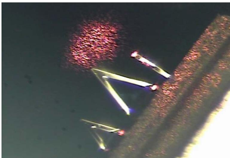
Figure 3. Rectangular PSI cantilever
