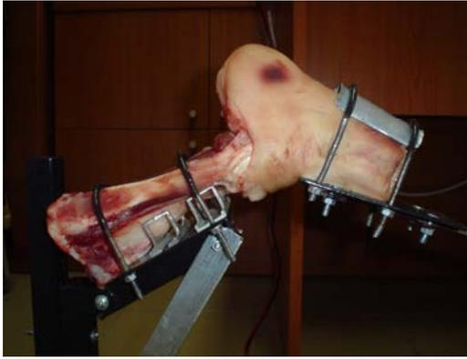
Figure 4. Joint clamped on the experimental apparatus [6]
