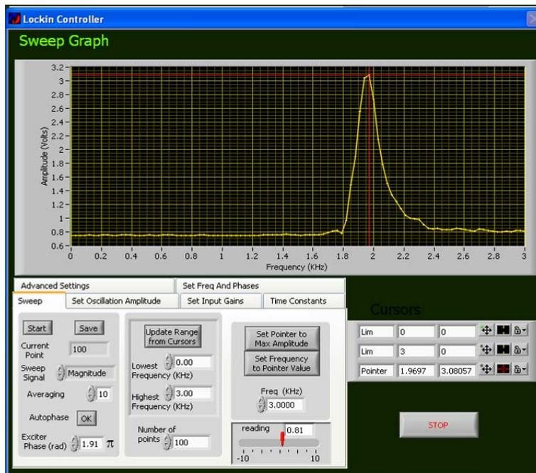
Figure 6. Frequency sweep curve of cantilever in T90 lubricant oil
